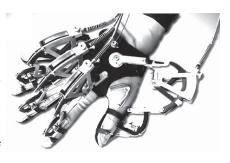
doing this uses fiber-optic cables stretched the length of each finger. Each cable has tiny cuts in it so, as you flex your fingers back and forth, more or less light escapes. A photocell at the end of the cable measures how much light reaches it and the computer uses this to figure out exactly what your fingers are doing.
