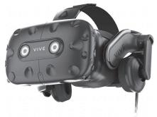
world), and stereo headphones. The two screens display slightly different, stereoscopic images, creating a realistic 3D perspective of the virtual world. HMDs usually also have built-in accelerometers or position sensors so they can detect exactly how your head and body are moving (both
